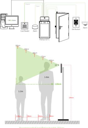
Recommended installation height: 150cm emperature Measurement Distance: 30cm~120cm
