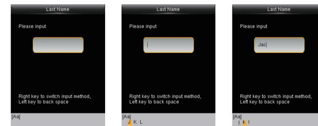
Press ► key to switch input methods: mixed case, upper case, lower Case, number and symbol.
