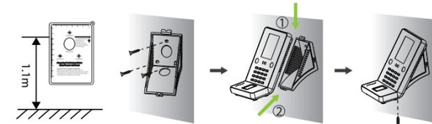
1. Post the installation template on the wall and drill. The distance from baseline to the ground is 1.1m by recommendation (for height in 1.55m to 1.85m). If the distance is 1.2m, the suitable height for users is beyond 1.65m.
