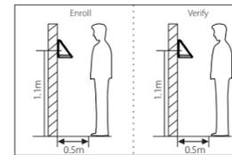
Recommended using methods (shown as left figures): During enrollment and verification, the installation position of device must remain the same. If need to move the device, keep the same installation height, or else, the recognition function will be poor.
